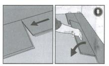
8. Place the panel gently and tight to the short end of the previous panel and fold it down in a single action movement.
