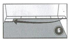
6. Second row First plank min length 500 mm. Put a distance against the wall.
